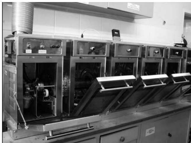
Figure 22. Continuous microwave reactor with rotating quartz tube for the synthesis of high-molecular-weight epoxy resin (Ertec, Poland).
